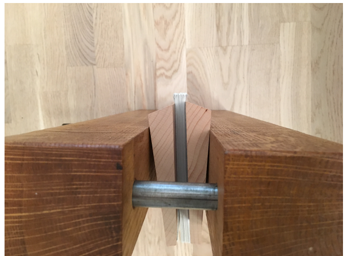
Fig. 3. Here you can see backing boards in a press.
