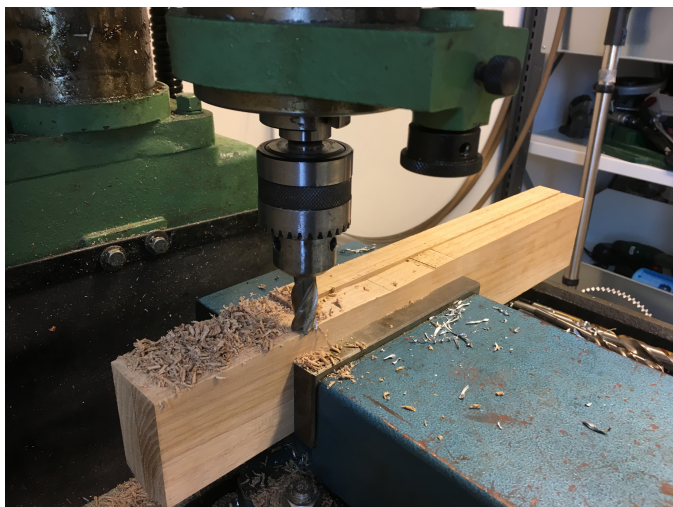
Fig. 9. Here you can see a the reducing of the wooden boards.
