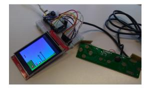
As noted earlier there are 12 buttons, but only 5 wires coming out of the gamepad. Those would be Vcc, Clock, Latch, Clock and Ground. Below is the image illustrating it. Image is taken from Hackaday article<sup>1</sup> about how to connect Snes controller to Arduino, but since the code is simple and self-explaining it is not hard to port it to ESP32 platform. The protocol used is already described in the article so I'm not going to repeat it again here.
