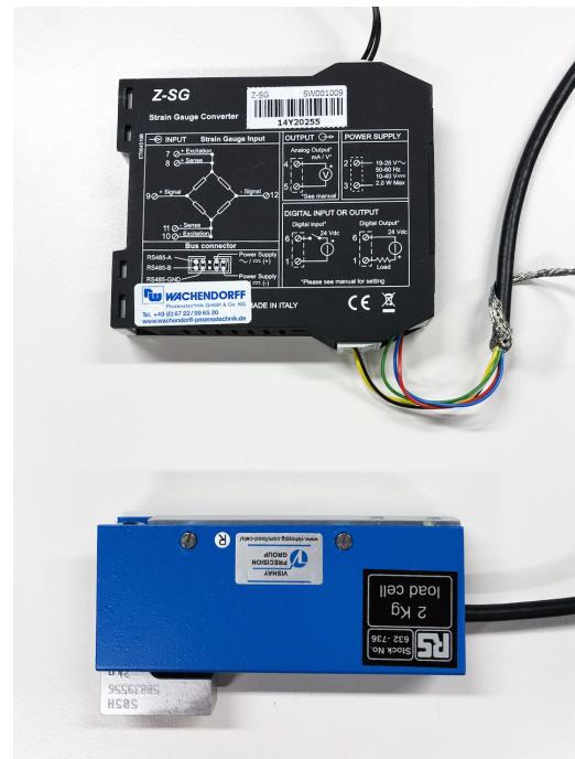
Fig. 6. Teda Hunteleigh Compression Load Cell (2kg), with a Wachendorff Strain Gauge Converter (11) (12).
