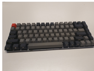
Fig. 1. Soldered switches with keycaps without walnut case
