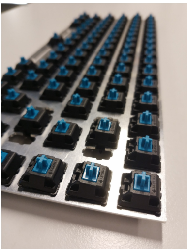
Fig. 4. Blue switches on aluminium plate
