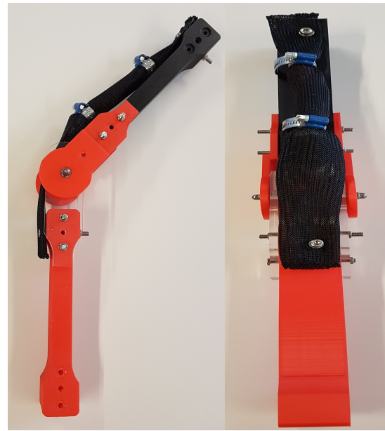
Fig. 8. Prototype robot joint constructed as part of IN5590 subject
