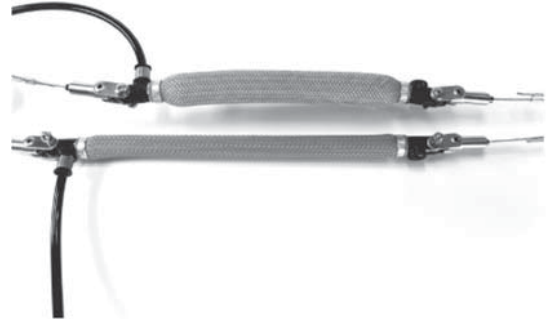
Fig. 1. McKibben actuator adapted from [18]
