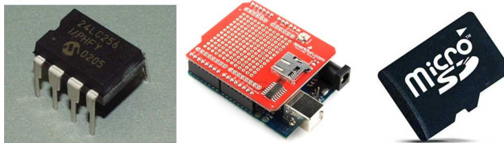
Figure C.3: Left to right : 1:External EEPROM memory | 2: MicroSD shield for Arduino boards | 3: microSD card
