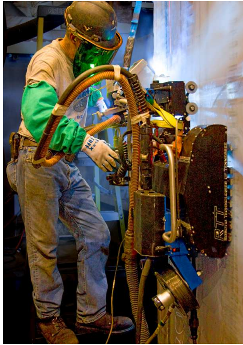
Figure 2.2: Operator works side by side with a climbing welding robot (on-site user).
