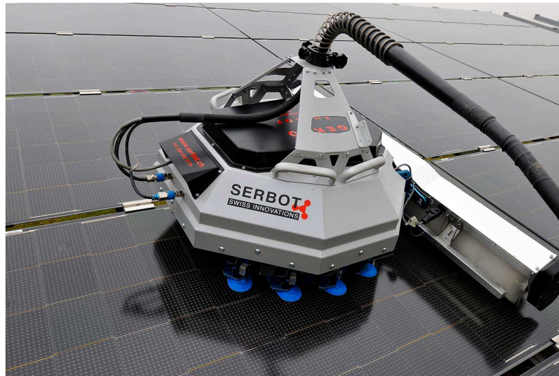
Figure 2.3: Autonomous cleaning climbing robot for glass and solar panels.
