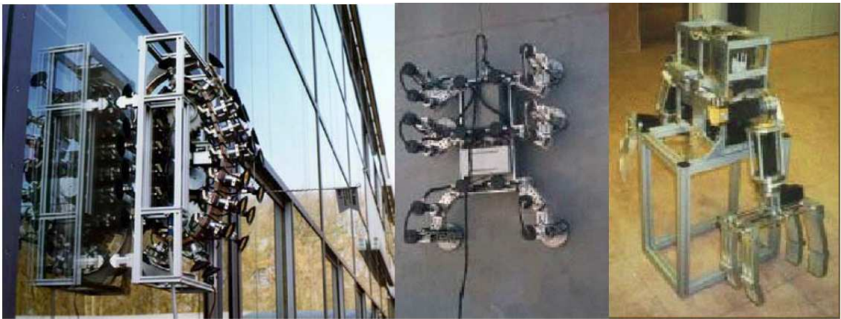
Figure 2.1: left to right Max V a chain-driven climber using vacuum cups, developed at University of Aalen - Rest six legged welding robot using magnetic force, Developed at CSIC Madrid - Roma grasping robot, specialized for inspection in steel bridge, developed at University of Madrid
