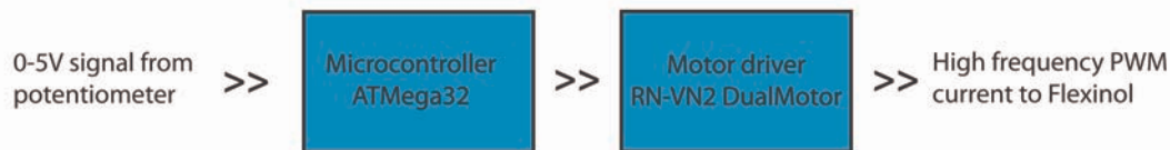
Figure 6.4: Block diagram of manual regulation. The voltage signal from the potentiometer is mapped directly to a pwm signal from the motor driver
