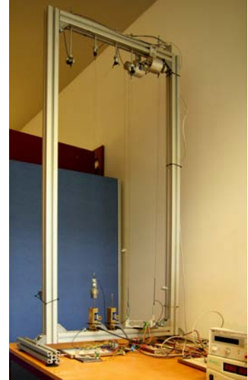
(b) A test frame was built to investigate the long term properties of Flexinol
