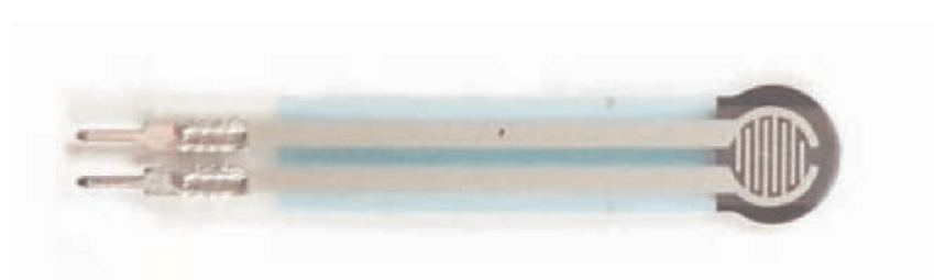
Figure 2.30: Interlink Force Sensing Resistor [67]. Small changes in pressure result in large changes in resistivity
