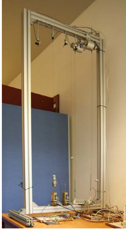
Figure 4.4: Developed test frame. Two radial displacement transducers are seen in the top and to linear displacement transducer are seen in the bottom. The frame holds 5 Flexinol wires in parallel
