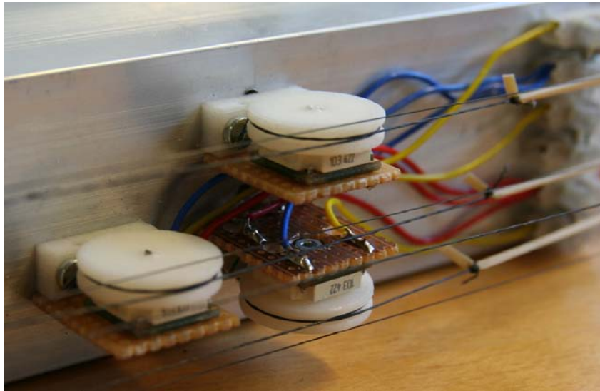
Figure 4.27: Radial displacement transducer mounted on the forearm. Rubber band and Flexinol wires can also be seen
