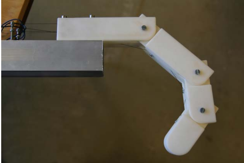
(a) Humanoid finger developed in this thesis. The finger is actuated with three Flexinol artificial muscle fibers and controlled with a microcontroller
