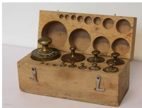
Figure 4.13: Calibration weights. Combinations of the weights are used to calibrate at 100g steps
