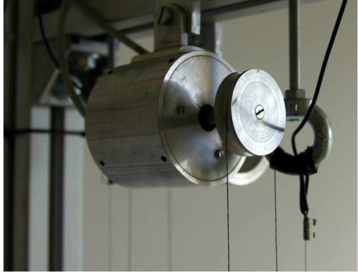
(b) Radial displacement transducer. A thread is routed over to wheel to measure displacements
